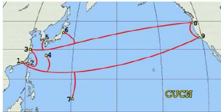
Figure 7: China-US Cable Network. 2000. The first un-dersea fiber optic cable network between US and China. [should be redrawn for the publication]
